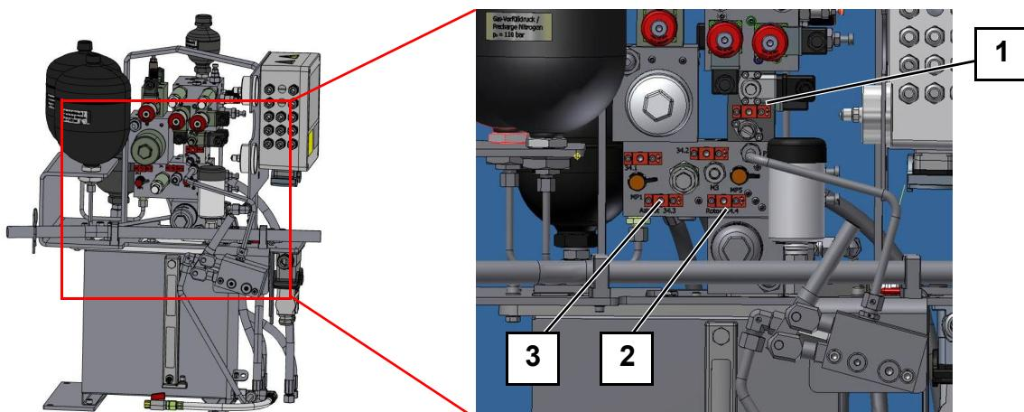
Abb. 23 Hydraulikaggregat Hawe
