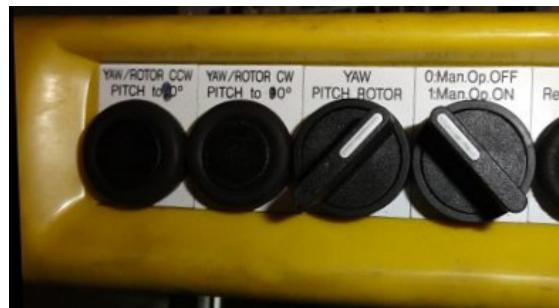
Abb. 27 Mobiles Bedienterminal
